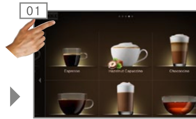
01 Switch to Maintenance level.
