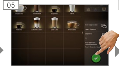
05 Start preparation of each of the products in the waiting list by pressing the green button.
